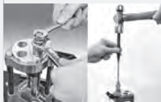
Lee Dies feature a Built-in Stuck Case Remover
