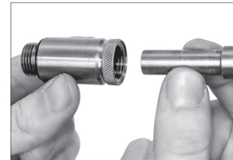
Install extension tube into body as shown
