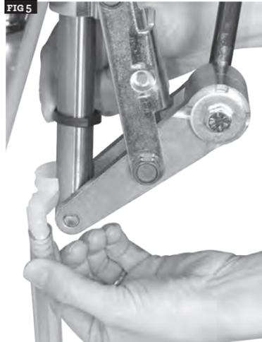
Slide retaining ring on to assembly.
