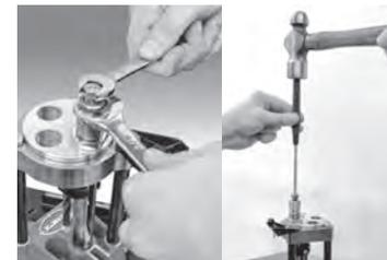
**Stuck Case** If a case is not lubricated, the rim will be pulled off and the case remains stuck in the die. If this happens — **loosen, but do not remove the decapper clamp with a 3/4" and 1/2" wrench.** Use a 3/16" drift punch and large hammer (1-lb. or larger) to tap on the decapper rod and drive the stuck case free. Lee Precision will remove a stuck case for \$6.00.
