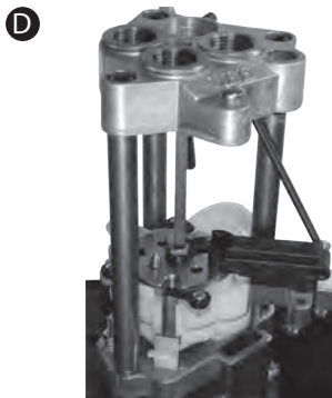
With the carrier at the bottom of the stroke (handle up), install index rod.
