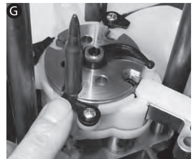
Push case retainer against case rim in each shell plate position
