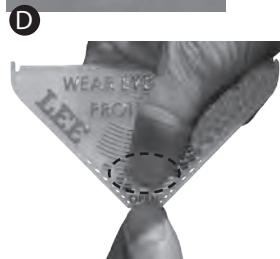
Fold cover over, slide the flow control to LOCK position, feel for the detent. Grasp the top and bottom of the flow control valve using your thumb and index finger above and below tray. NOTE: make sure it is in the LOCK detent position, else primers may spill.
