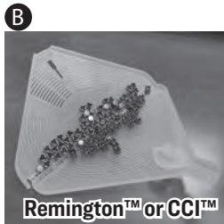
Fold cover over, slide the flow control to LOCK position, feel for the detent. Grasp the top and bottom of the flow control valve using your thumb and index finger above and below tray. NOTE: make sure it is in the LOCK detent position, else primers may spill.
