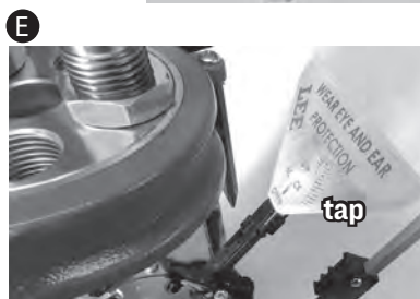
Slide the tray into the trough. Slide the flow control to the ON position. Tap the side of the tray several times to fill the trough.
