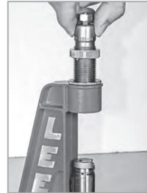
**2 INSTALL SIZING DIE** If cost is more important than convenience, you can leave the quick change bushing permanently installed after installing the sizing die. While holding the handle against the stop, screw the die in until it touches the shell holder, then release pressure from the handle and screw in the die in additional 1/4 to 1/2 of a turn maximum. Now while holding the die, tighten the lock ring. **NOTE:** Carbide dies should not be screwed in the additional 1/4 to 1/2 turn.
