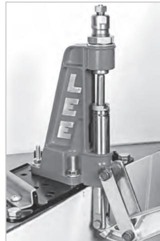
**4 PLACE LUBRICATED CASE** in the shell holder and raise the ram until the handle comes to a stop. Lower the ram and remove case.
