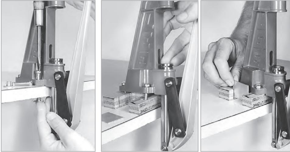
**ATTACH** your press with (3) 1/4" bolts. Use 'T' nut for quick removal to empty spent primers. **NOTE** You may drill a hole through the bench and catch the primers in a container below.
