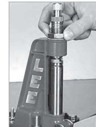
**8 SCREW** the bullet seating die in until you feel it touch the case mouth. If no crimp is desired, back the die out 1/2 turn. If a crimp is desired, turn the die in 1/4 turn.
