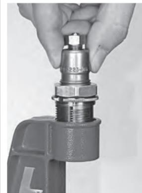
To remove quick-change bushing, rotate the die 1/6 of a turn counterclockwise, lift out. You can add bushing to your next die, or install an additional bushing on the rest of your dies for quick-change convenience.
