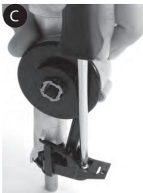
**C:** Re-install 6-32 Phillips screw to secure disconnector.
