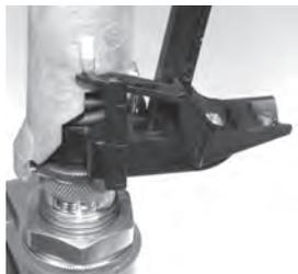
Disconnector and latch lever installed.
