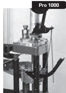
**D** Lower the ram while lifting the loose end of the bead chain. The beads will snap through the disconnecter and rest in the proper position.
